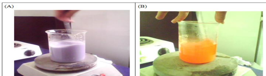
Fig. 1. Sample Pictures for A) Cooking of Bioplastics from Indigenous Plants and B) Cooked Starch Solution Ready for Molding
